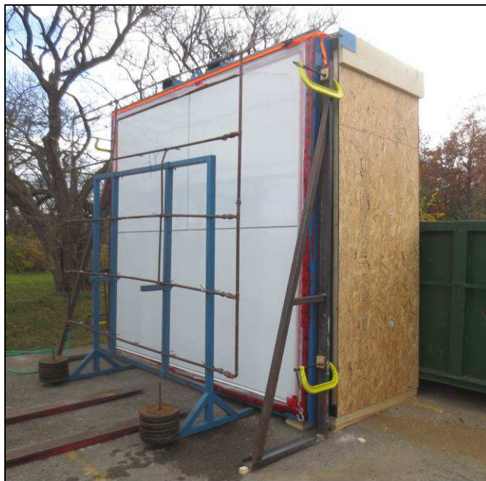
Figure C2 - Spray rack Set up for water penetration
